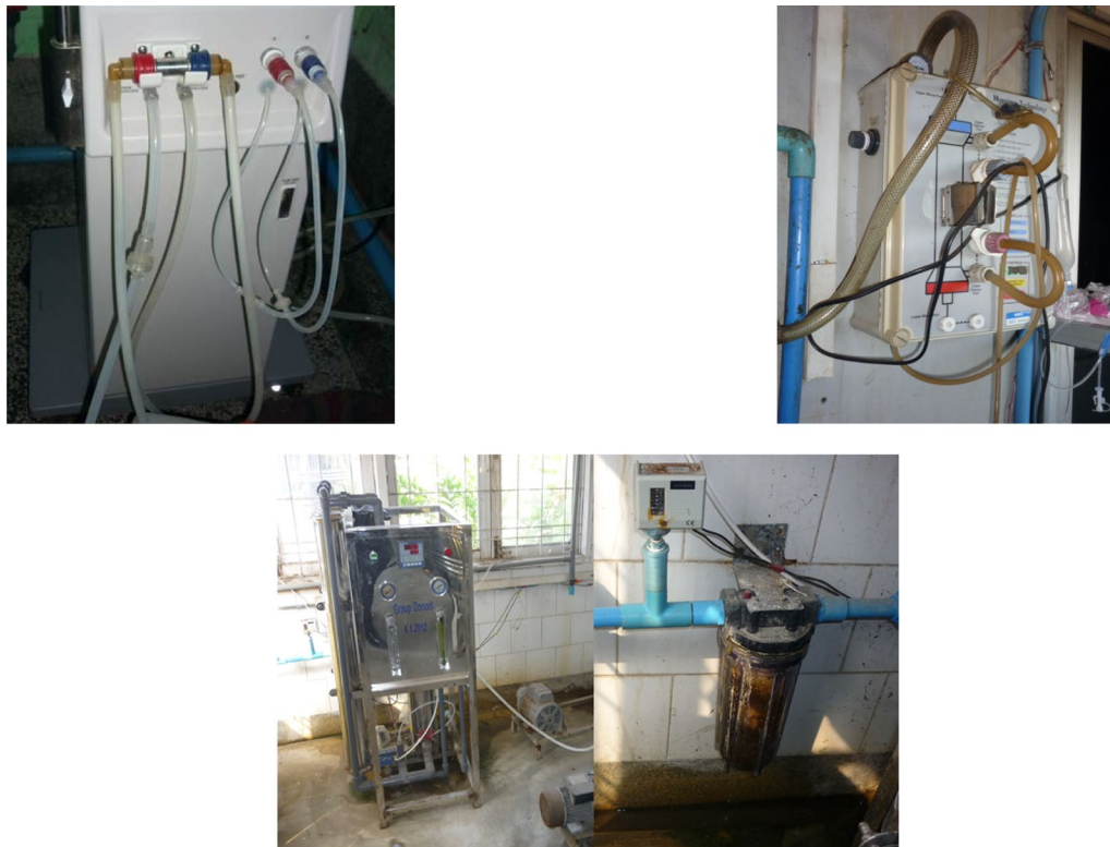
Fig. 2 The dialysis machines were very dirty and in poor condition because they had been gifted by an international organization and the local hospital did not have staff capable of maintaining them
