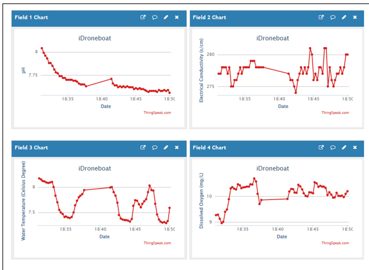
Fig. 5. An example of ThingSpeak's Graphical User Interface shows water quality data (pH, water temperature, EC, and DO).
