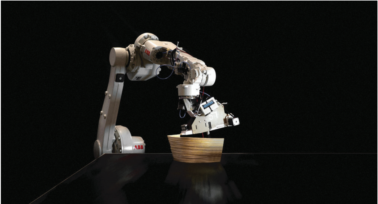
FIG. 9. Printing result of the multilayer lamination technique. The flexibility of the willow material also enables curvature printing, as examined in Ref. 46 We identified a minimum radius of 20 mm for in-plan curvature and a maximum overhang angle of 22.5^\circ for the printing of larger parts of walls.
