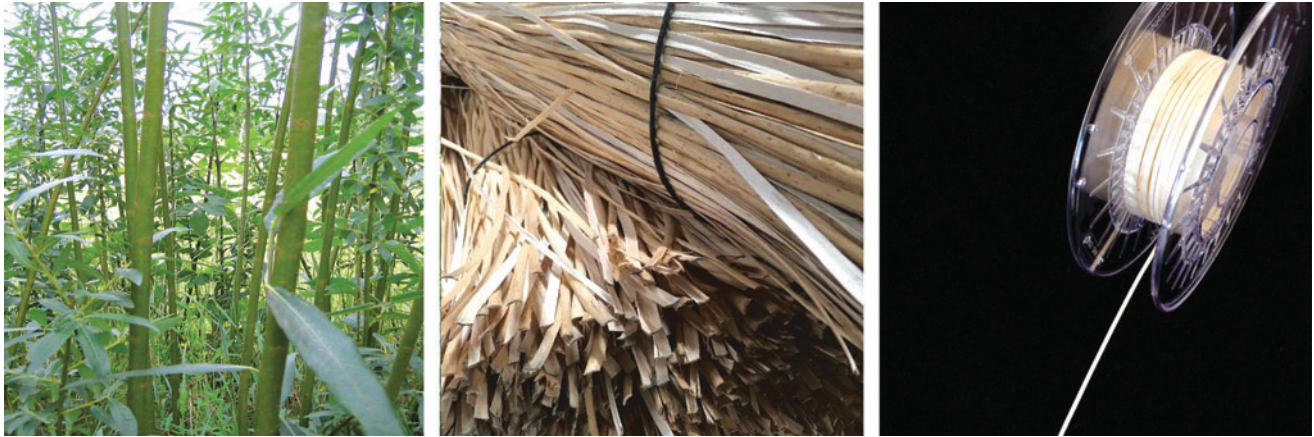
FIG. 1. (Left) Willow twig plantation of “ Salix Americana ” genus: The twigs can be harvested in 1-year cycles. (Middle) The outer shell of the harvested twigs is split in multiple strips after harvesting. (Right) Continuous, solid willow filament rolled on a regular 3D printing spool.
