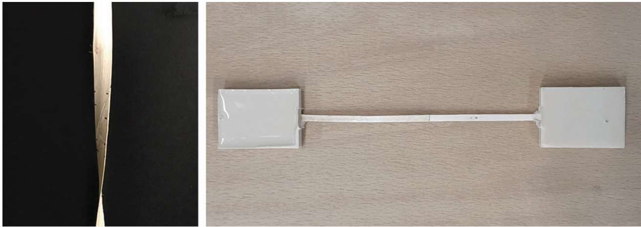
FIG. 2. (Left) The filament joint with an angled cut to maximize the surface area for adhesives. (Right) Specimen ends were embedded in casting resin to prevent defects by clamping into the test machine.
