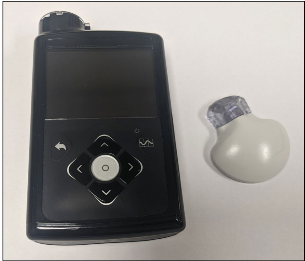
Fig. 1 Medtronic 670G insulin pump (left) with Guardian Sensor 3 continuous glucose monitor (right)
