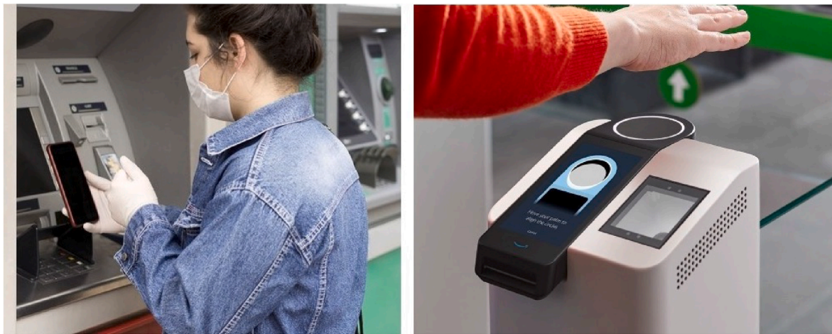
Fig. 7. (i) Cardless ATM machine, providing touchless interaction with smartphone by scanning a QR code to establish connection [33] (ii) Amazon One palm detection as touchless technology for access control [34].
