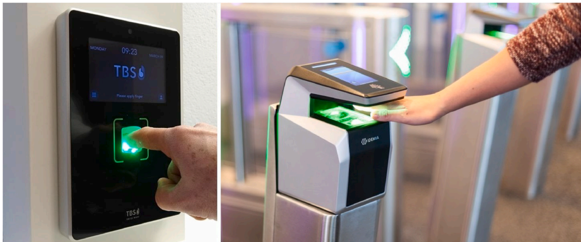
Fig. 3. (i) Touchless biometric finger scan [15] (ii) Hand scanning as access control to workplaces [16].
