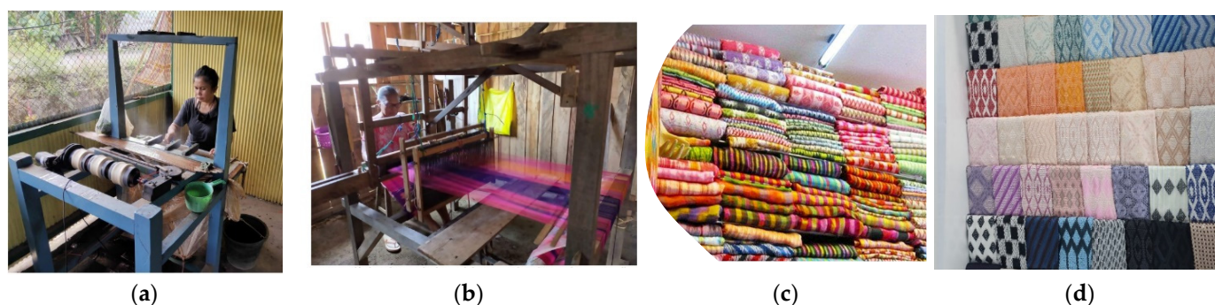
Figure 6. Process and material fabrics. (a) spinning; (b) weaving; (c) Sulawesi woven fabrics; (d) West Java woven fabric.
