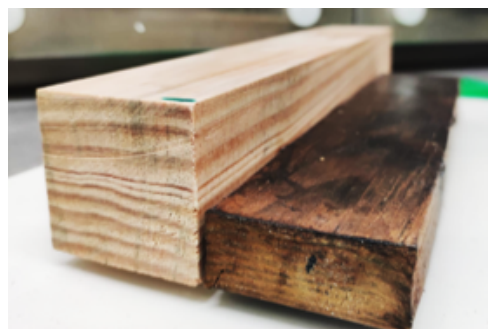
Figure 7. Visual comparison between a natural block and a densified block (with mould).
