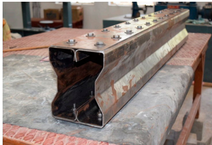
Figure 8. CFS beam specimens before testing cold-formed built-up sections.
