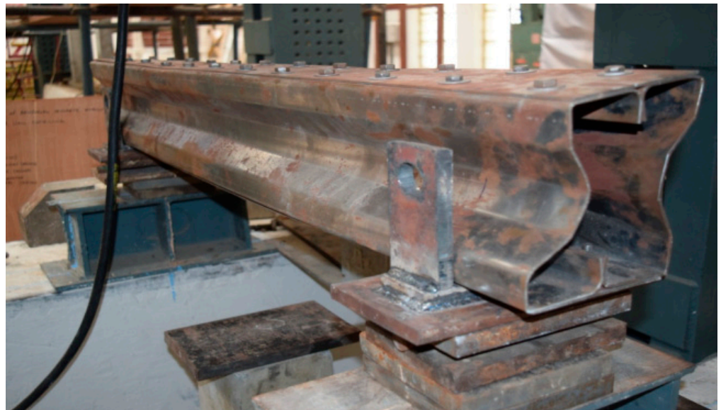
Figure 10. The failure mode of F2F100.
