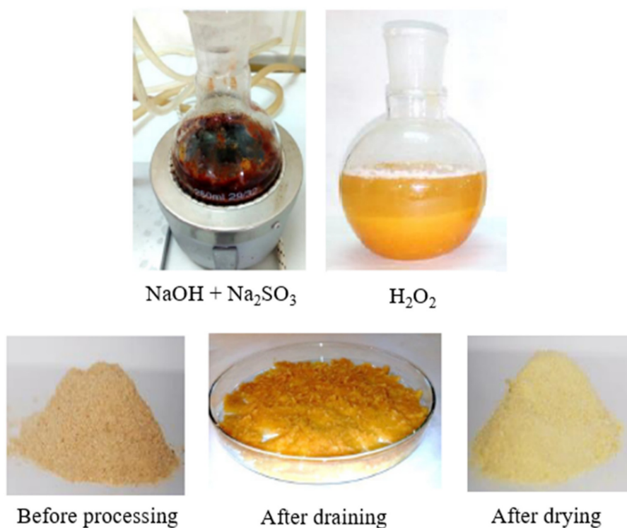
Figure 4. Stages of chemical modification.
