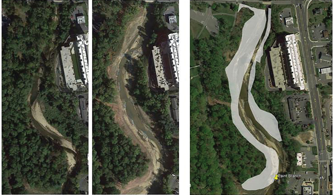
Figure 2: Tree removal at Paint Branch during stream restoration. Before (2012) After (2014)
