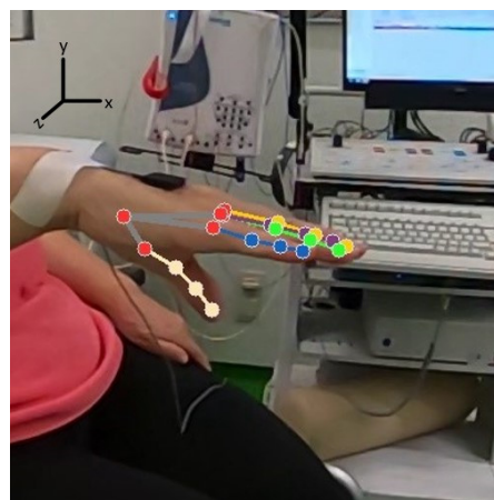
Figure 2. Example landmarks extraction process (beige: thumb, lilac: index finger, yellow: middle finger, green: ring finger, blue: little finger, red: wrist, carpometacarpal and metacarpophalangeal joints).
