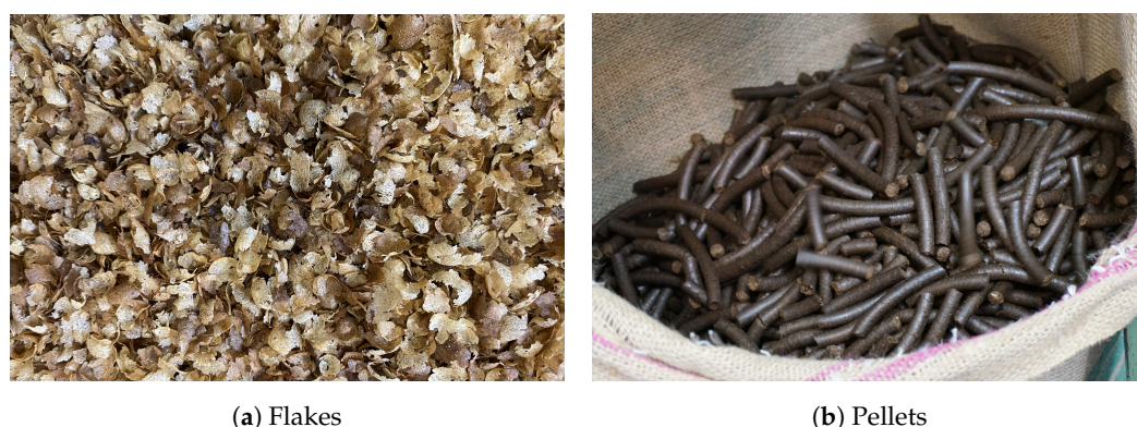
Figure 2. Processed silver skin. (a) Silver skin as flakes. (b) Silver skin pressed into pellets. (Photos by the authors).
