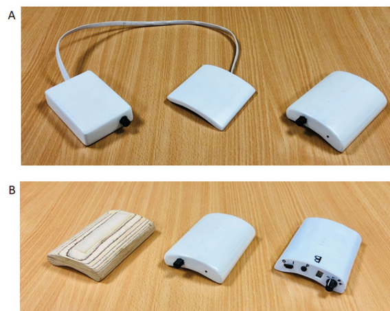
Figure 4. Models created for pre-pandemic usability studies of showing different shapes and forms for the stimulator (A). Models incorporating different control options were later produced (B) [40].
