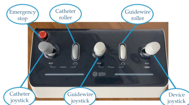
Figure 2 Control unit of ETcath200 robot-assisted system.
