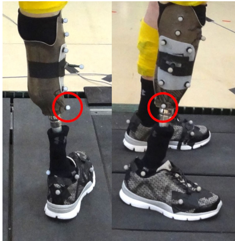
Figure 3. Static trial images showing the placement of the pylon marker. This marker is used in scaling the model to separately scale the residual limb and pylon segments
