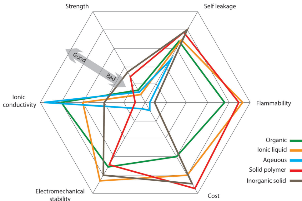
Figure 8. Comparison of the performance of several electrolyte types.
