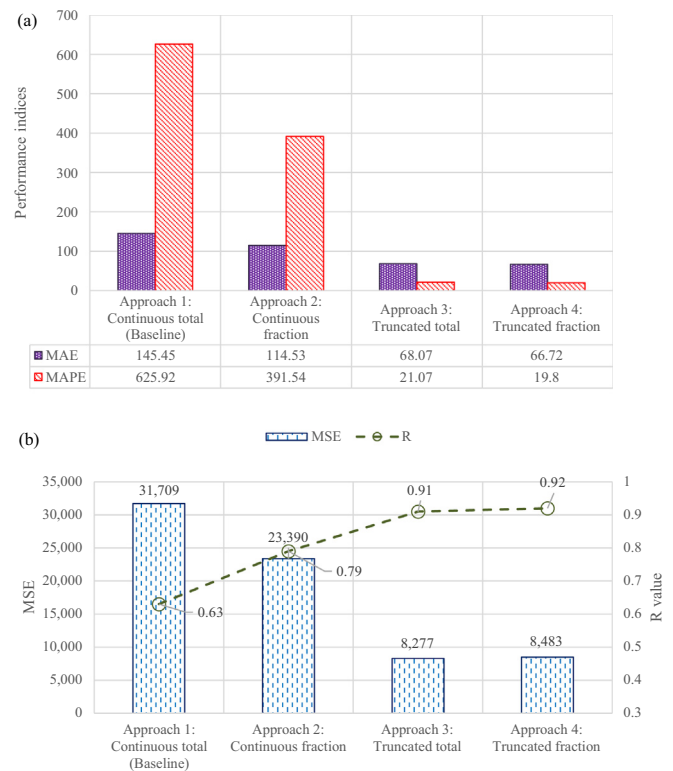
Fig. 3. Model performance comparison among Approach 1 - Continuous total (Baseline), Approach 2 - Continuous fraction, Approach 3 - Truncated total, and Approach 4 - Truncated fraction a) mean absolute error (MAE) and mean absolute percentage error (MAPE); b) mean square error (MSE) and R value.
