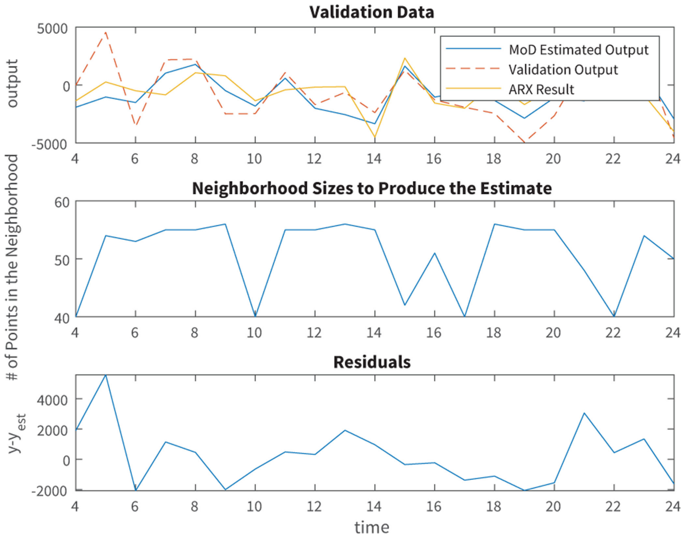
Fig. 2. MoD and ARX Models on Validation Data (25% of Participant Data). The output is measured in steps.
