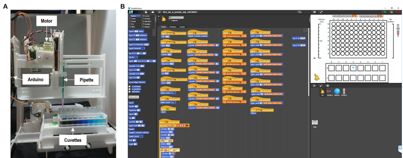
Fig 1. An open-source low-cost liquid handling robot (LHR) for STEM education and life-science experimentation featuring a block-based programming language. A) The main frame of the robot is made of laser-cut plastic parts, while all consumables (i.e. syringes, pipette tips, cuvettes, and well-plates) are standard life-science plastic ware that can be purchased online. B) The LHR interface was programmed in Snap4Arduino. (See also Supplementary Movies and reference [21]).
