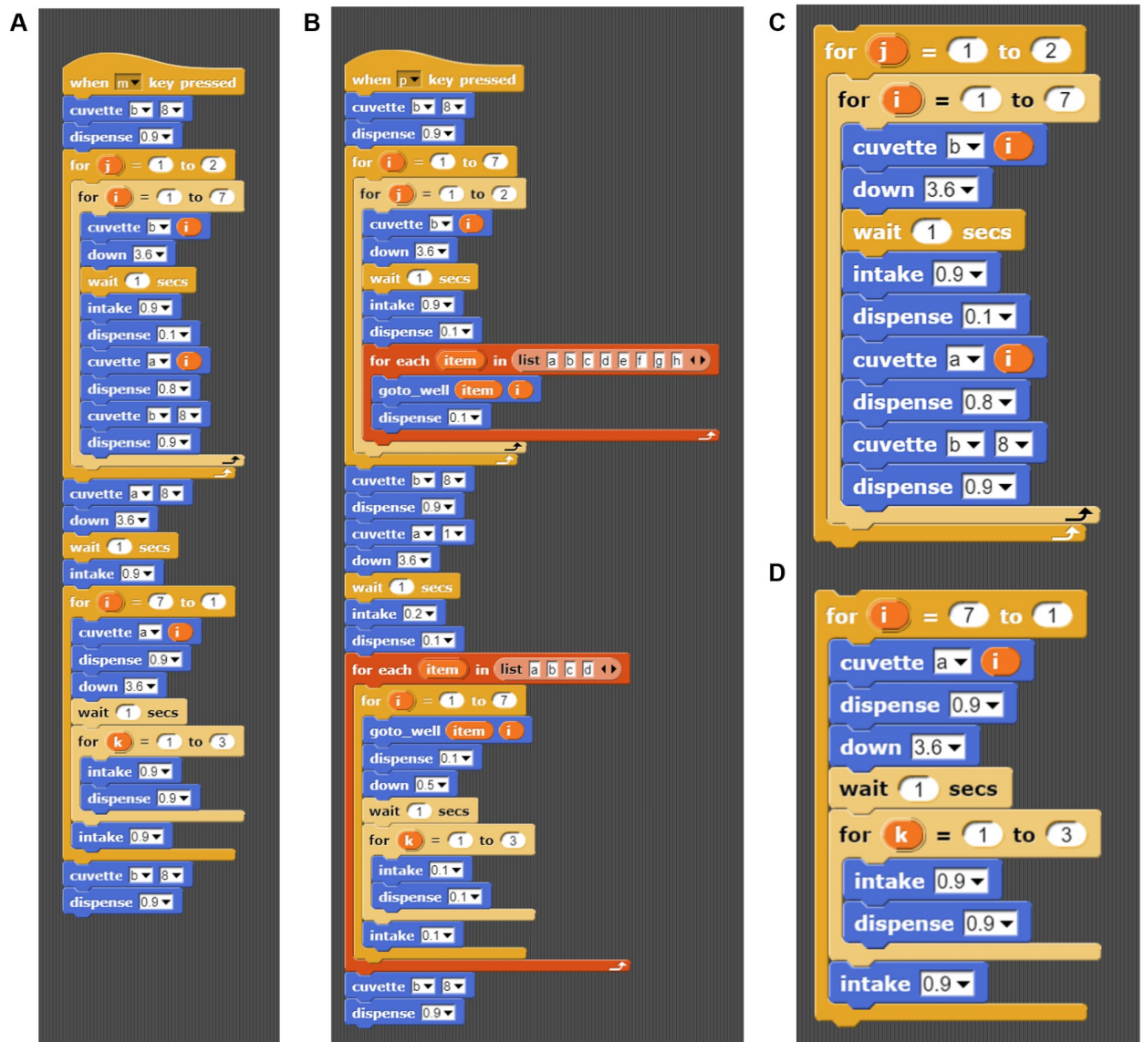
Fig 5. Examples of protocols featuring loops and iterative liquid handling operations. A) Serial dilution program for cuvettes. B) Serial dilution program for four rows of a 96-well plate. C) Zoom in of the first for-loop of the serial dilution program for cuvettes, which encapsulates the second for-loop. Note that the variables are marked in orange, the robot commands are marked in blue, and the for-loop visually encapsulates the entirety of its body. D) Third for-loop which encapsulates the fourth for-loop of the serial dilution program for cuvettes.
