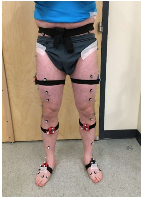
Figure 2. IMU and reflective marker placement for human subject experiments.
