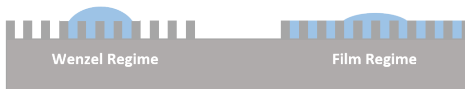
Figure 7. Schematic of water droplet behaviors on a rough hydrophilic surface.
