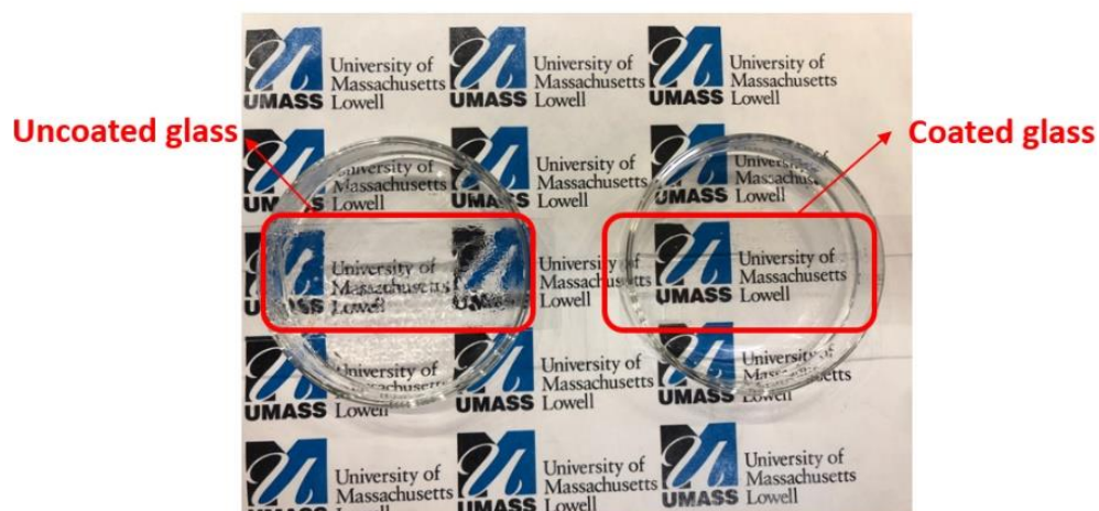
Figure 10. Bare glass (left) and SS6 coated glass (right) holding over a glass Petri dish containing hot water.
