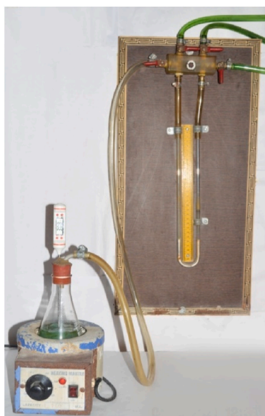
Fig. 5. Arrangement to heat the mixture of pyrolysis oil and plastic waste.
