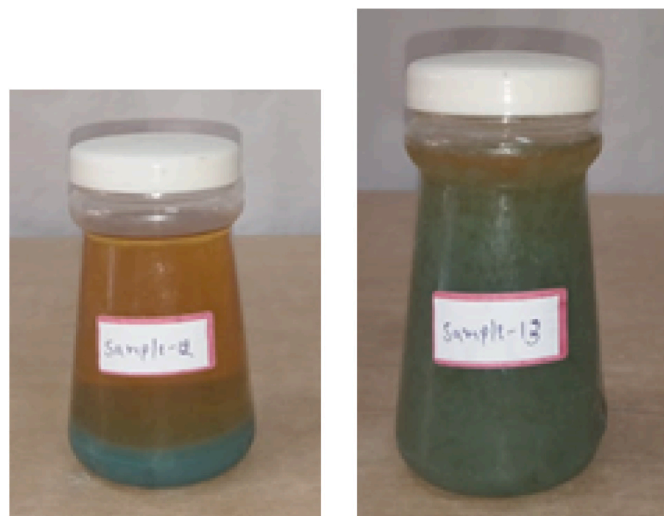
Fig. 16. Solutions of LDPE + HDPE solvent after the dissolution of plastic mask for samples 12 and 13.
