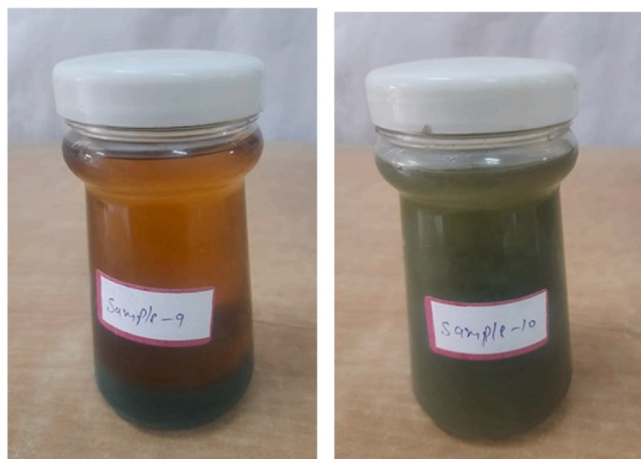
Fig. 12. Precipitation of dissolved facemask for samples 9 and 10 in ascending order of heating rate.
