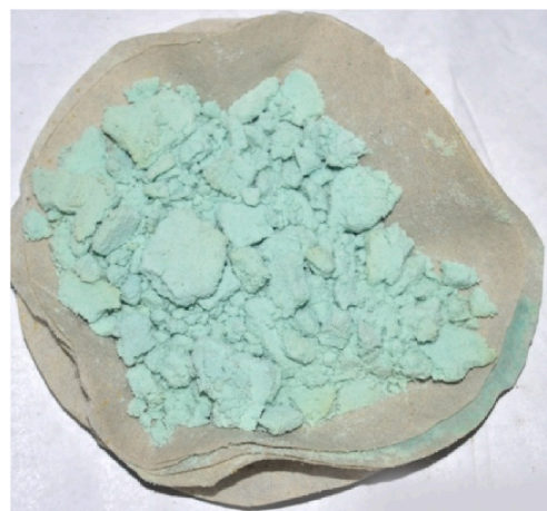
Fig. 17. Powder form of dried precipitate of the dissolved facemask for sample 8 (PP + PE oil).
