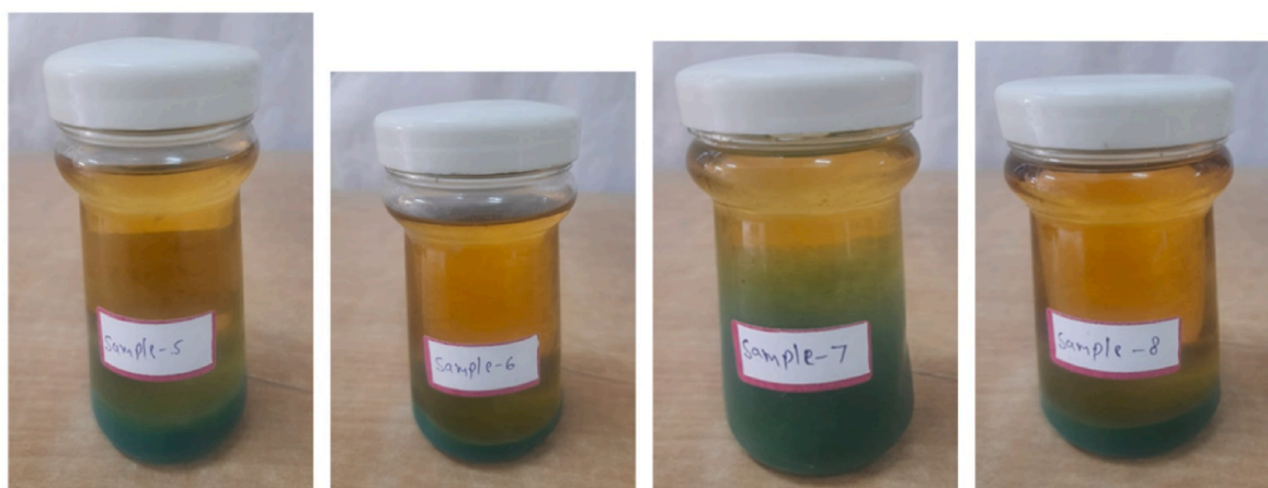
Fig. 10. Precipitation of dissolved facemask for samples 5–8.
