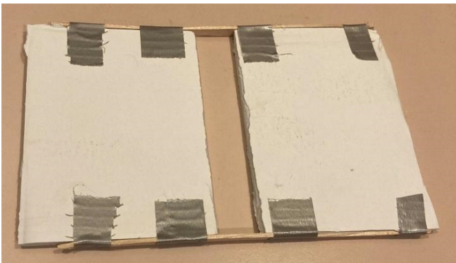
Figure 3. Setup testing platform This figure illustrates the testing platform used to aid in the isolation of the signal. The gap in the center of the platform kept the Petri dish off the surface of the table. This ensured the dish did not touch the testing table and further suspended the mycelial bridge in midair.
