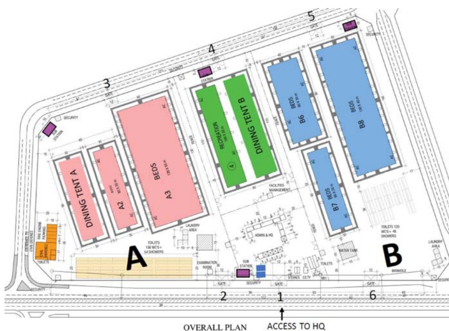
Figure 1. Layout of the temporary isolation tent camp.
