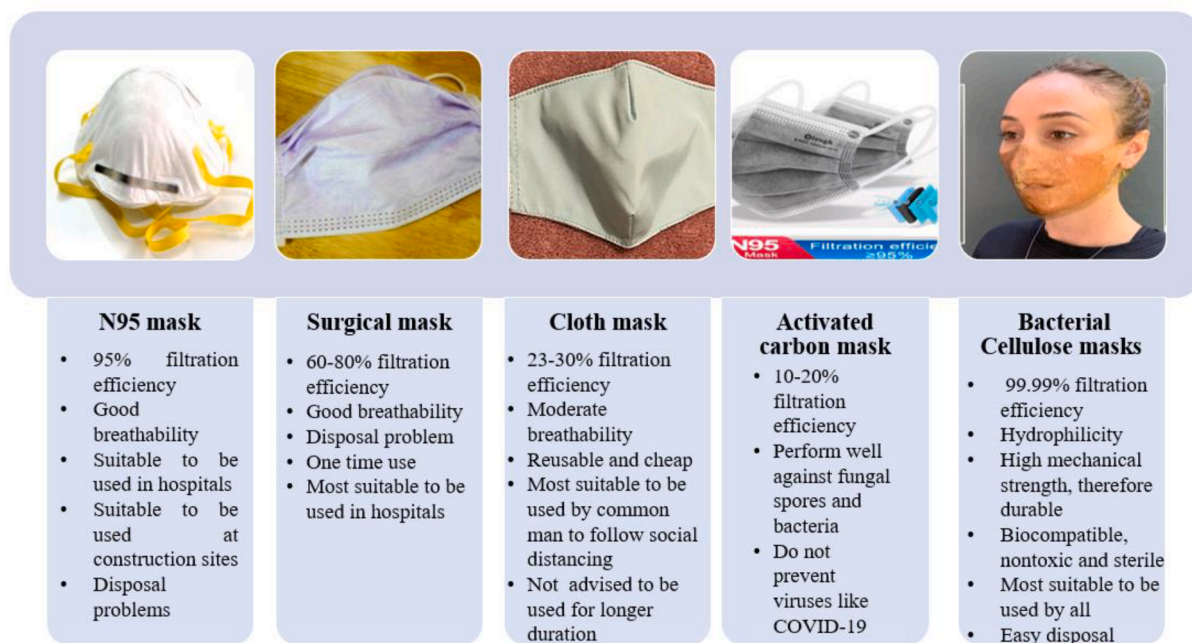
Fig. 3. Comprehensive features of different types of conventional masks (such as N95 mask, surgical mask, cloth mask, activated carbon mask) and biodegradable mask (bacterial cellulose mask) (Gope et al., 2020; Gustafsson et al., 2018).
