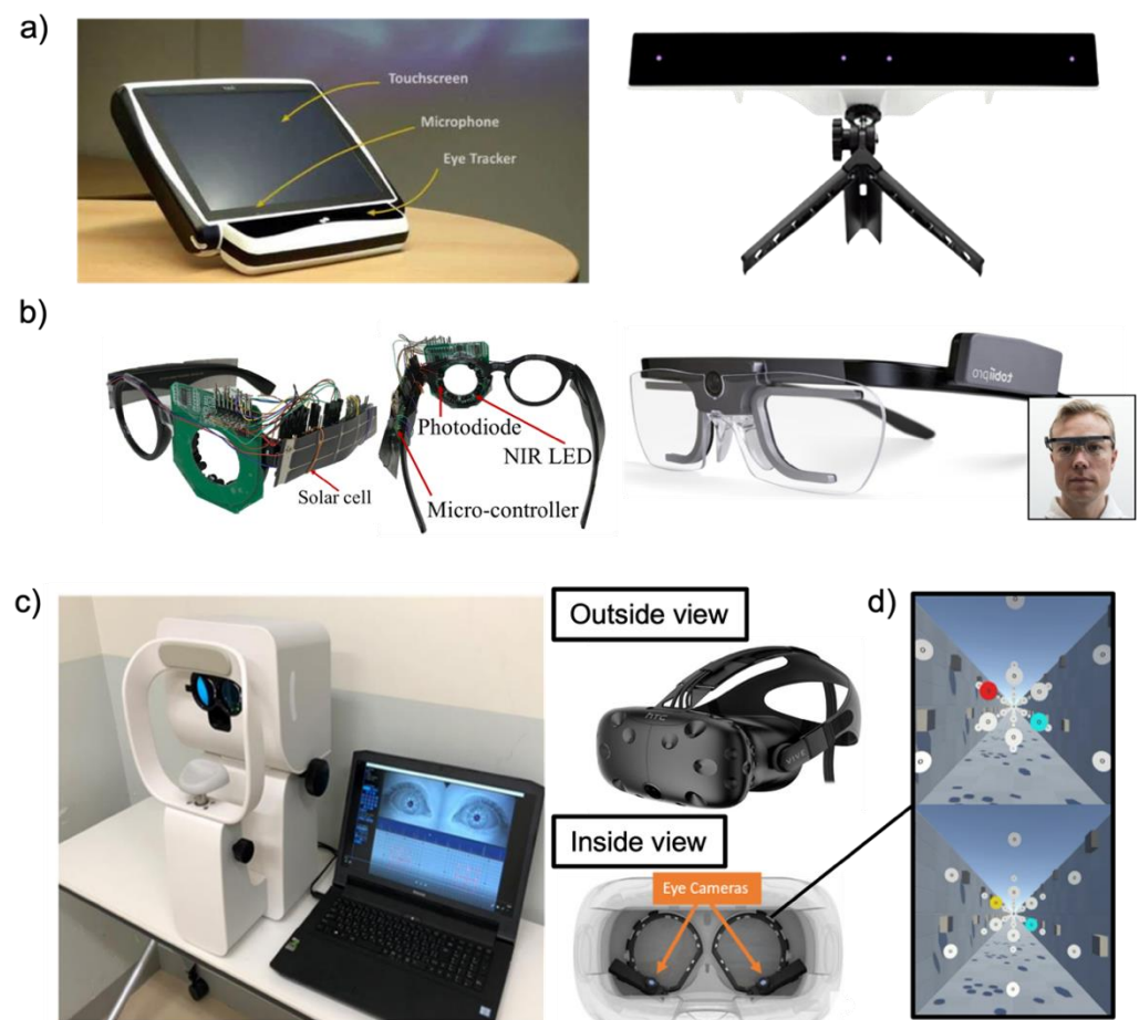
Figure 14. Eye tracking platforms. (a) Glass-type eye tracker (Left: Reprinted with permission [184]. Copyright 2013, Springer-Verlag London, Right: Reprinted under terms of the CC-BY license [3]. Copyright 2020, the authors. Published by MDPI). (b) Screen-based eye tracker (Left: Reprinted with permission [174]. Copyright 2022 ACM, Inc., Right: Reprinted under terms of the CC-BY license [160]. Copyright 2020, the Authors. Published by Springer Nature). (c) VR hardware platform (Left: Reprinted under terms of the CC-BY license [182]. Copyright 2020, the Authors. Published by DOAJ., Upper right: Reproduced under terms of the CC-BY license [3]. Copyright 2020, the Authors. Published by MDPI, Lower right: Reproduced under terms of the CC-BY license [183]. Copyright 2020, the Authors. Published by DOAJ). (d) Perceptual depth change with eye trackers in virtual reality (Reprinted under terms of the CC-BY license [177]. Copyright 2021, the authors. Published by Frontiers).
