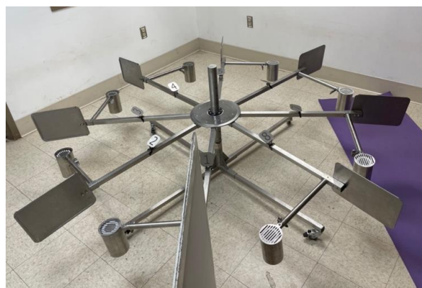
Figure 1. A photo of the 8-port scent wheel used in this study.
