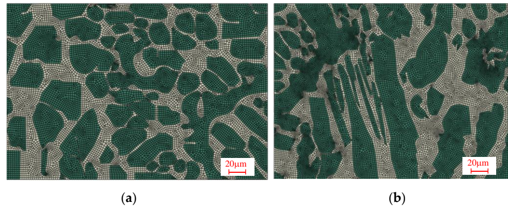
Figure 4. Geometric model and meshing of representative regions: (a) uniform area of grain ellipse (1#) and (b) vertically fenced area (2#).
