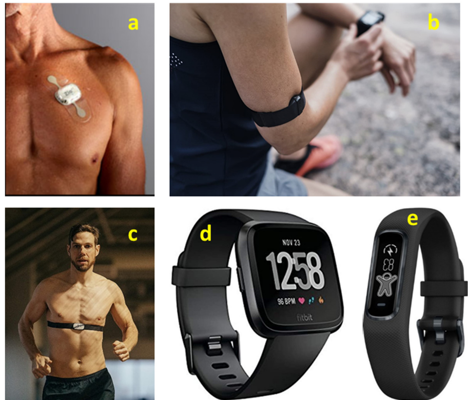
Figure 8. Examples of wearable cardiac monitors. (a) iRhythm ZIO AT chest patch monitor (medical grade, https://www.irhythmtech.com , accessed on 17 August 2022), (b) Polar OH1 upper arm band monitor ( https://www.polar.com/us-en , accessed on 17 August 2022), (c) Wahoo TICKR X chest strap ( https://www.wahoofitness.com , accessed on 17 August 2022), (d) FitBit Versa smart watch ( https://www.fitbit.com/global/us/home , accessed on 17 August 2022), (e) Garmin VivoSmart 4 wrist strap monitor ( https://www.garmin.com/en-US , accessed on 17 August 2022).
