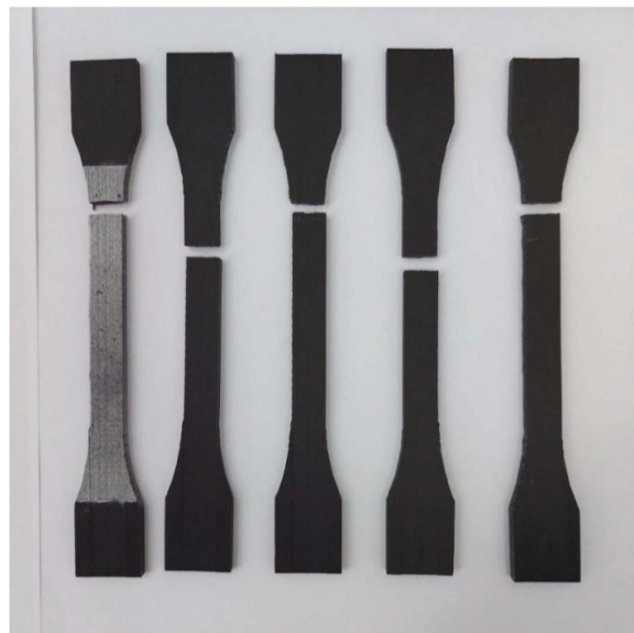
Figure 14. Failure mode of the XY specimens.
