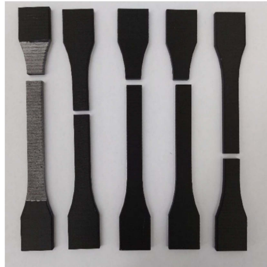
Figure 16. Failure mode of the XZ2 specimens.
