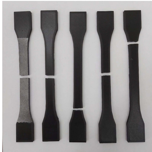
Figure 12. Failure mode of the XZ1 specimens.
