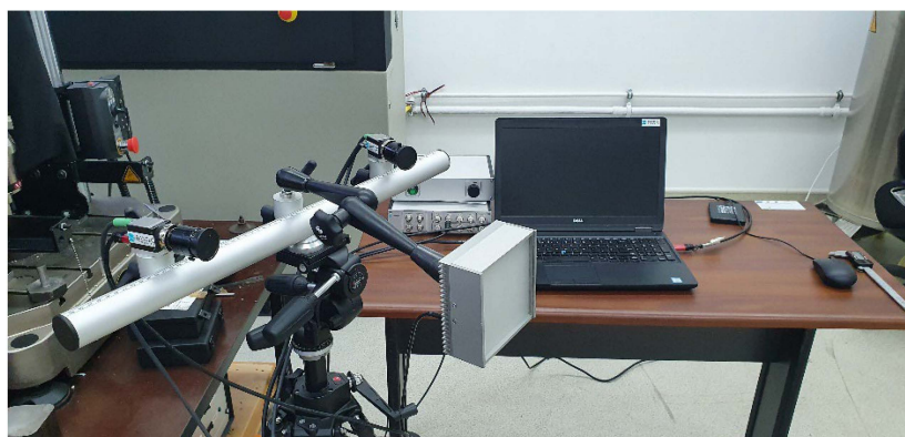
Figure 2. The Q400 Digital Image Correlation setup.
