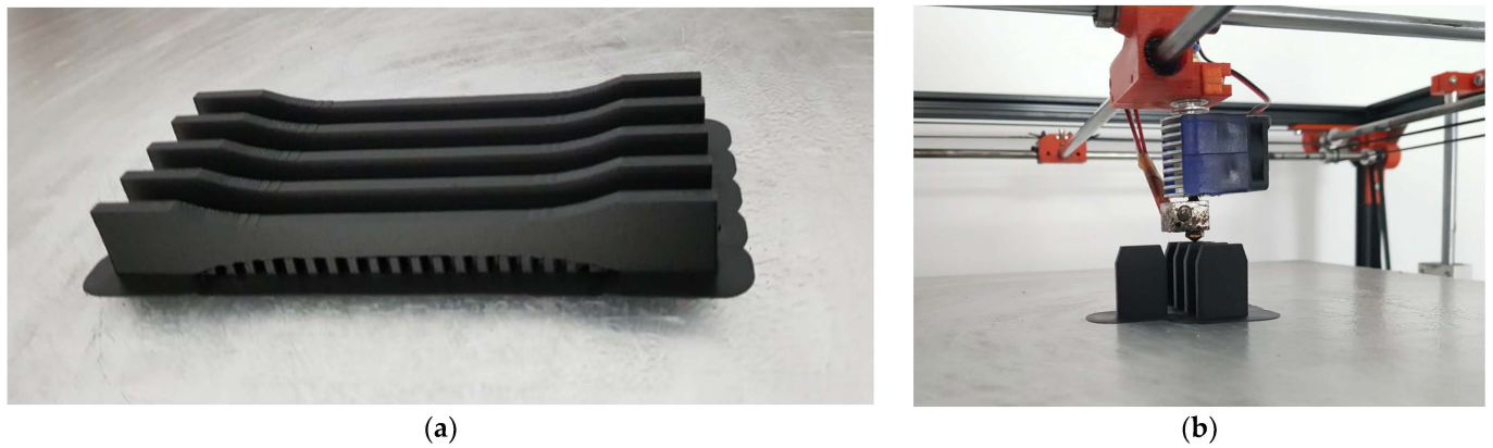
Figure 3. Different phases in the manufacturing process: (a) Tensile specimens printed on the lateral side, with overhangs; (b) Tensile test specimens printed along the vertical direction.
