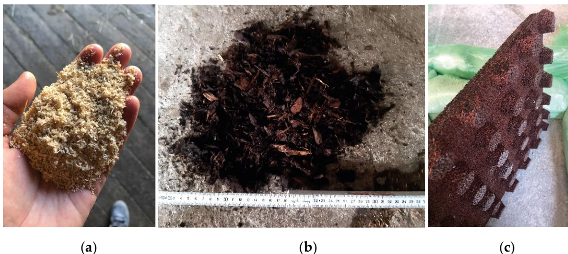
Figure 4. Three tested materials: sawdust (SAW) (a), bark mulch (BM) (b), and the soft rubber mat II (SRM II) (c). The rubber mat is presented from the lower side to display the rubber feet.
