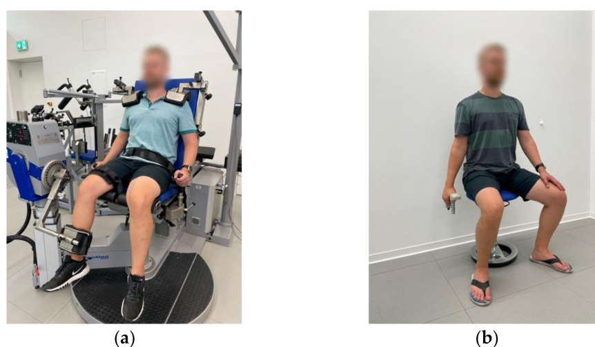
Figure 2. Correct positioning of participants during maximal voluntary contractions (MVC). (a) Kneec extension MVC of the right leg with IsoMed-2000 dynamometer; (b) handgrip MVC of the right hand with Jamar ® dynamometer.
