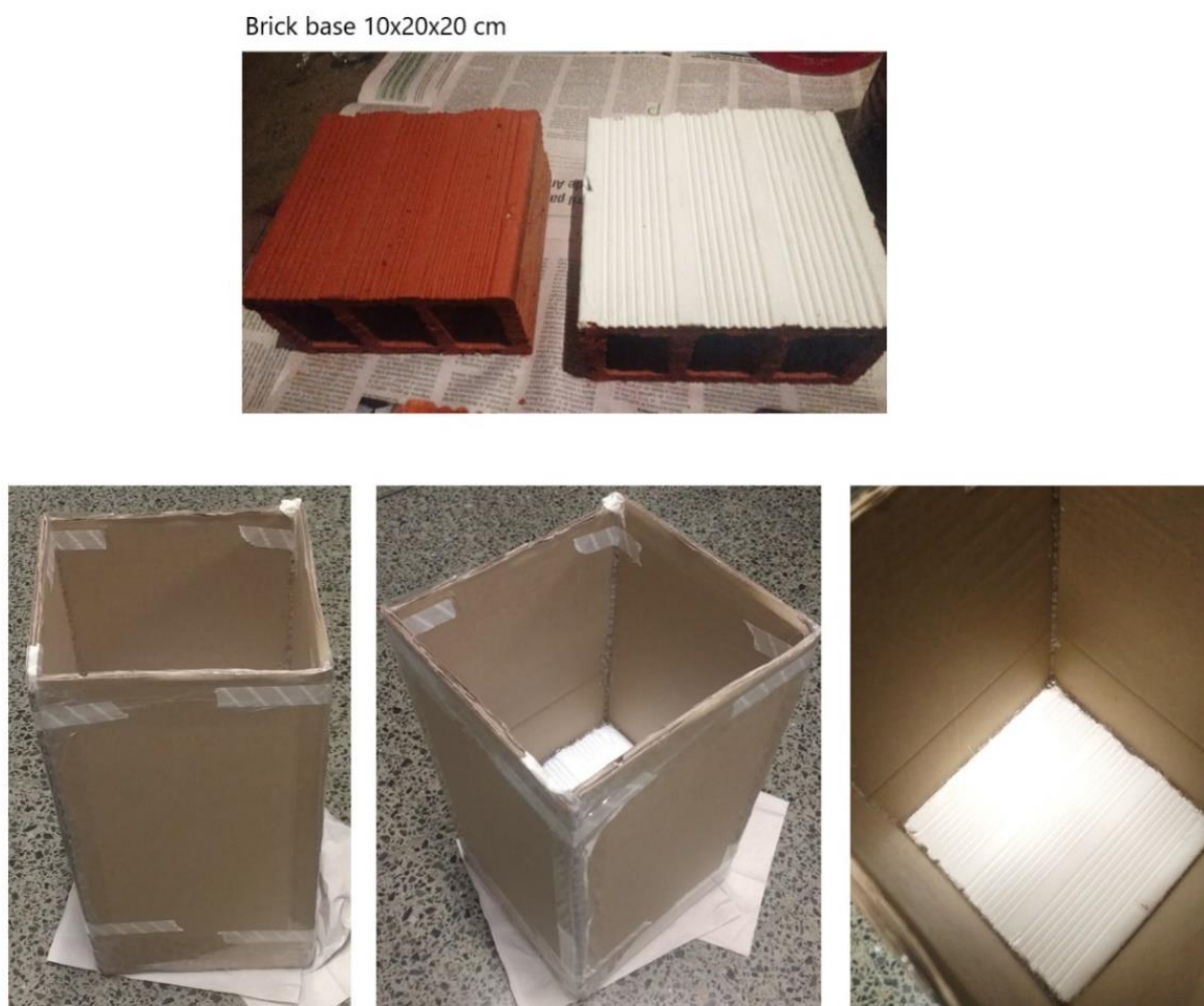
Figure 2. Bioassay prototype chambers for triatomine exposure to micro-encapsulated insecticidal paint. Triatomines were exposed for 1 h inside the chambers for follow-up at 24–48 h post exposure.
