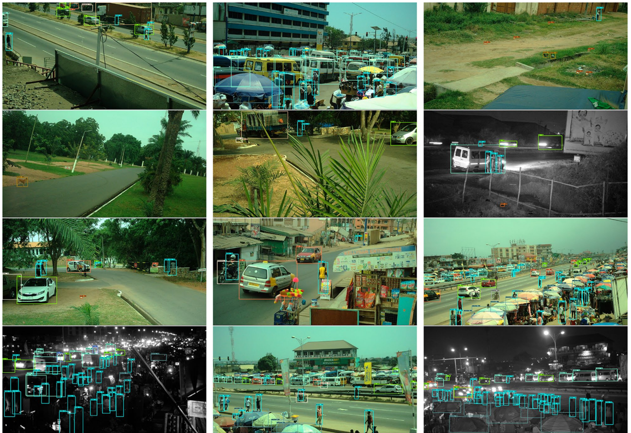
Figure 2. Objects identified in example images. Each identified object is bounded by a box, coloured by object type. The number next to the object's name shows the final layer's activation score for the given object's classifier, which may be heuristically interpreted as the network's confidence score in its prediction. "Truck" refers to pick-up truck, "Bowl" refers to cooking bowl/pot, "Stall" refers to market stalls and "Stove" to cookstoves of the type found in markets.
