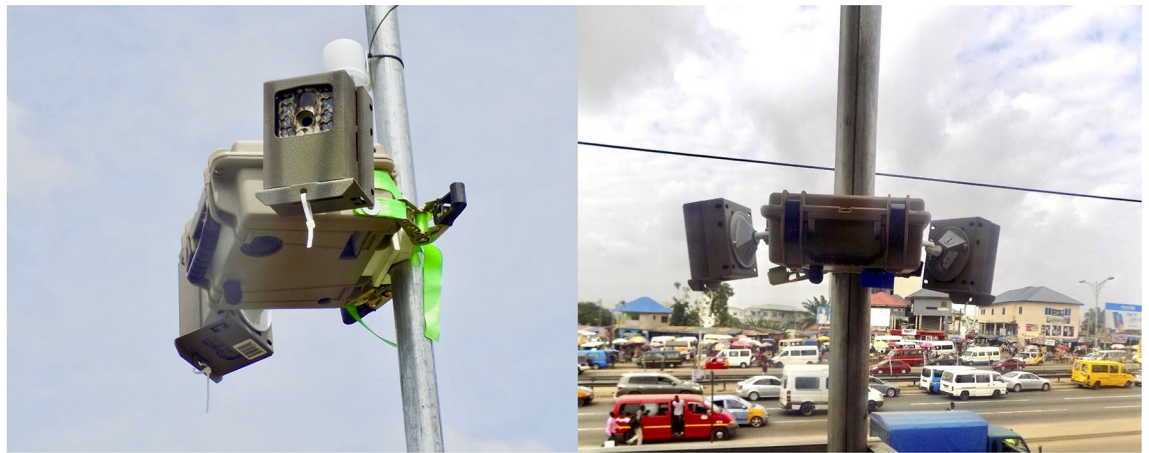
Figure 1. Examples of cameras used for image capture and their installation at measurement sites.
