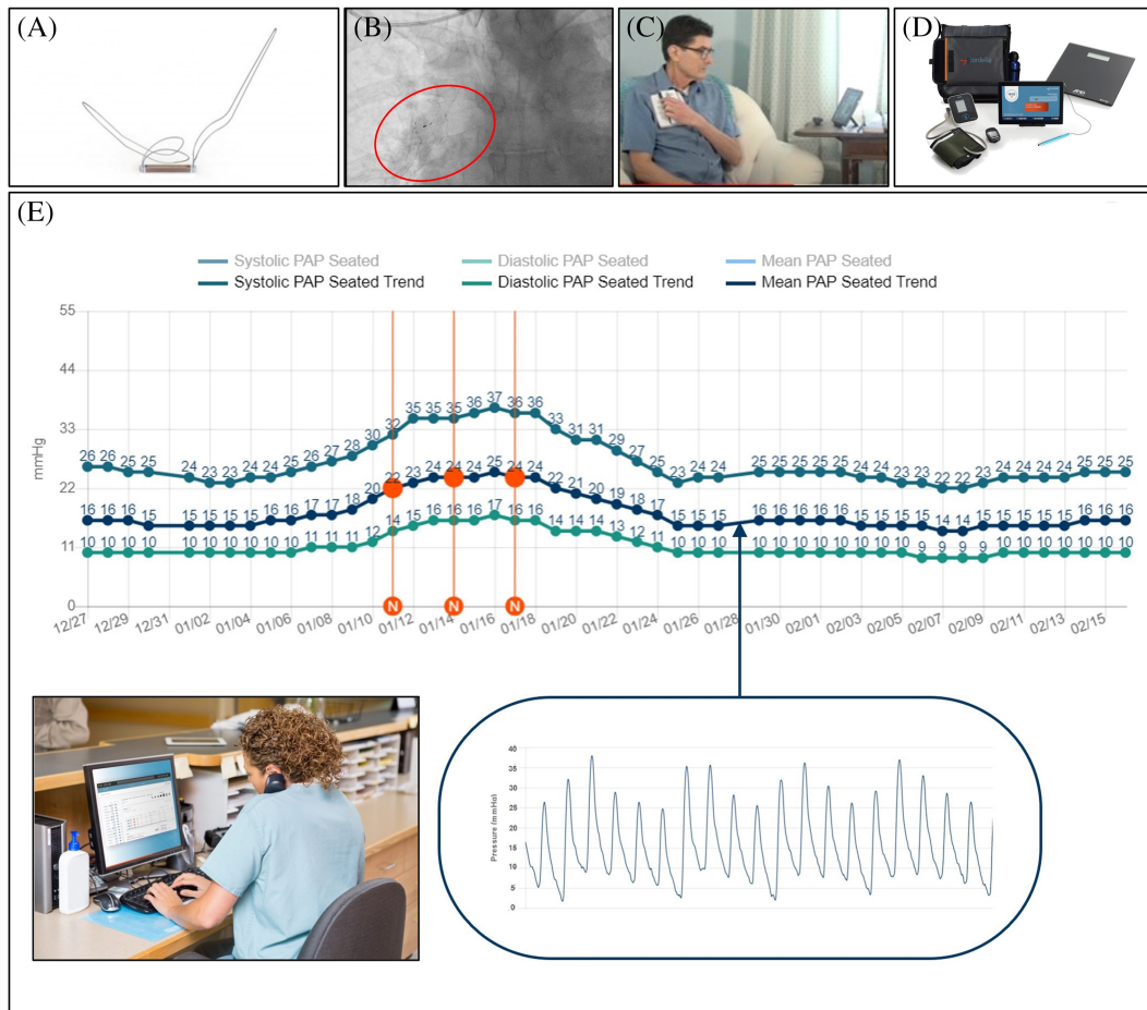
Figure 1 (A) Cordella pulmonary artery sensor. (B) Pulmonary angiogram depicting sensor deployment in the right pulmonary artery. (C) Depiction of patient using the handheld myCordella patient reader to measure seated PAP in the home environment. (D) Cordella patient kit with vital sign peripherals. (E) Cordella pulmonary artery pressure system trend waveforms as seen by the clinician through the patient management portal (PMP). The red vertical lines represent clinician notes. (Inset) Daily reading of mean pulmonary artery pressure. Respiratory fluctuations and secondary features such as the dicrotic notch are evident.
