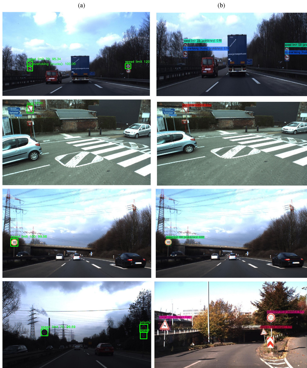
Figure 9. A comparison of the results from Faster R-CNN and YOLOv4. The first column (a) is from Faster R-CNN and the second column (b) is from YOLOv4. From the first row, Faster R-CNN misses the No overtaking sign and falsely classifies Speed limit 120 as speed limit 70 . YOLOv4 correctly detects and classifies all the signs. From the second row, Faster R-CNN miss classifies give way sign as bend sign . YOLOv4 correctly classifies the give way sign . From the third row, both Faster R-CNN and YOLOv4 correctly classify the speed limit 100 traffic sign . The last row shows how Faster R-CNN result in low light and YOLOv4 results in bright light. Both the models perform well in conditions of low light and bright light.
