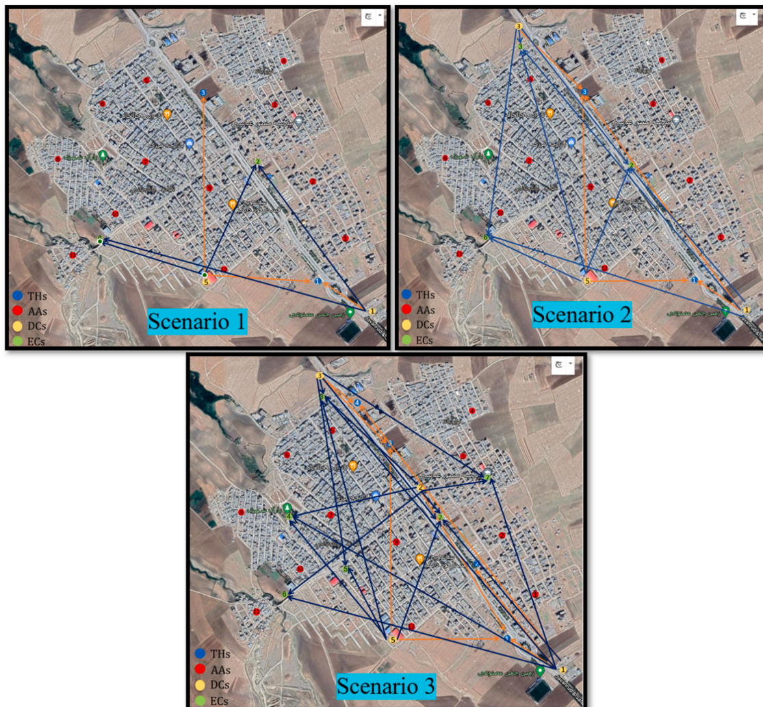
Fig. 10. The flow of RIs in three different scenarios (green arrows illustrate the flow between DCs and THs and yellow arrows define the flow for ECs). (For interpretation of the references to colour in this figure legend, the reader is referred to the web version of this article.)
