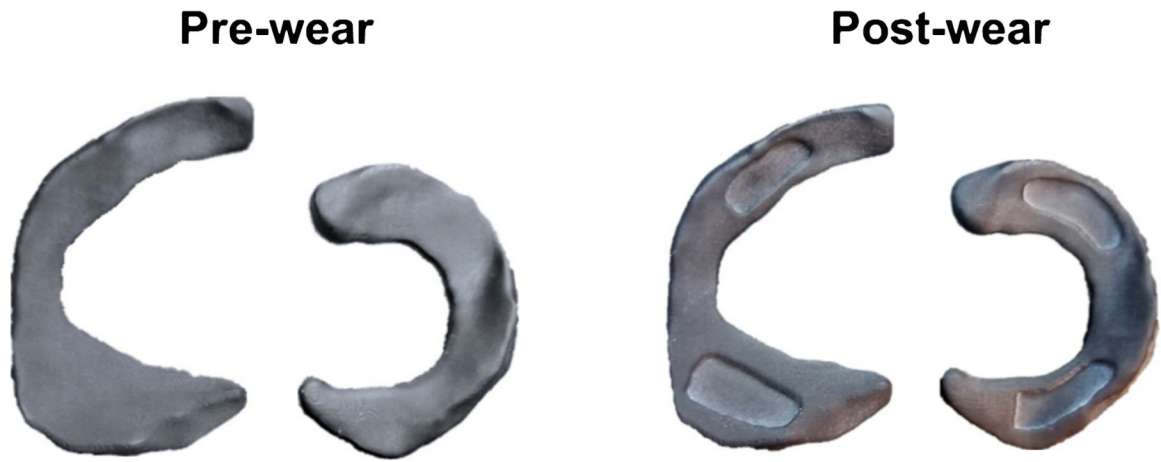
Fig. 3. Complex surrogate models were fabricated by 3D printing an MRI reconstruction of a healthy human menisci (pre-wear) and generating defects in the surface (post-wear). Images above are photographs.
