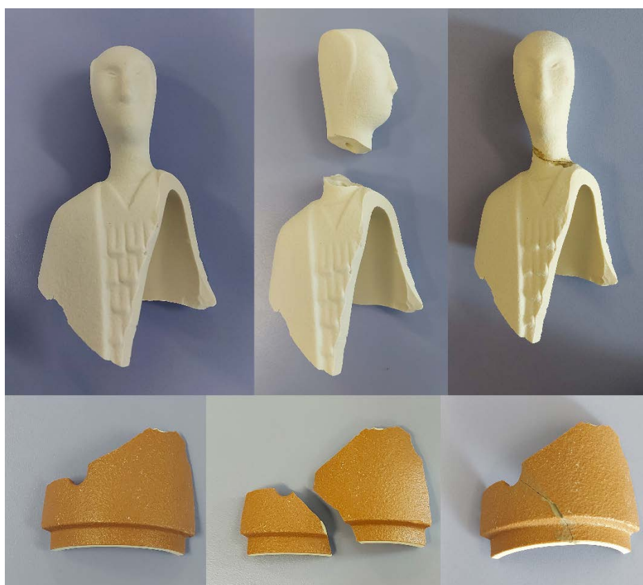
Figure 5. Porcelain stoneware and pottery artworks restored and repaired by using the geopolymer-based materials PS-MK and RP_{dry} -MK described in this paper.
