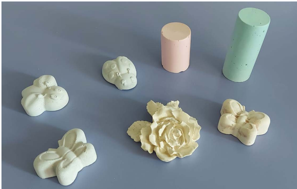
Figure 7. Examples of coloured artefacts created with the geopolymer-based materials described in this paper. As apparent, even objects with complex shapes can be easily realized by a simple casting procedure.
