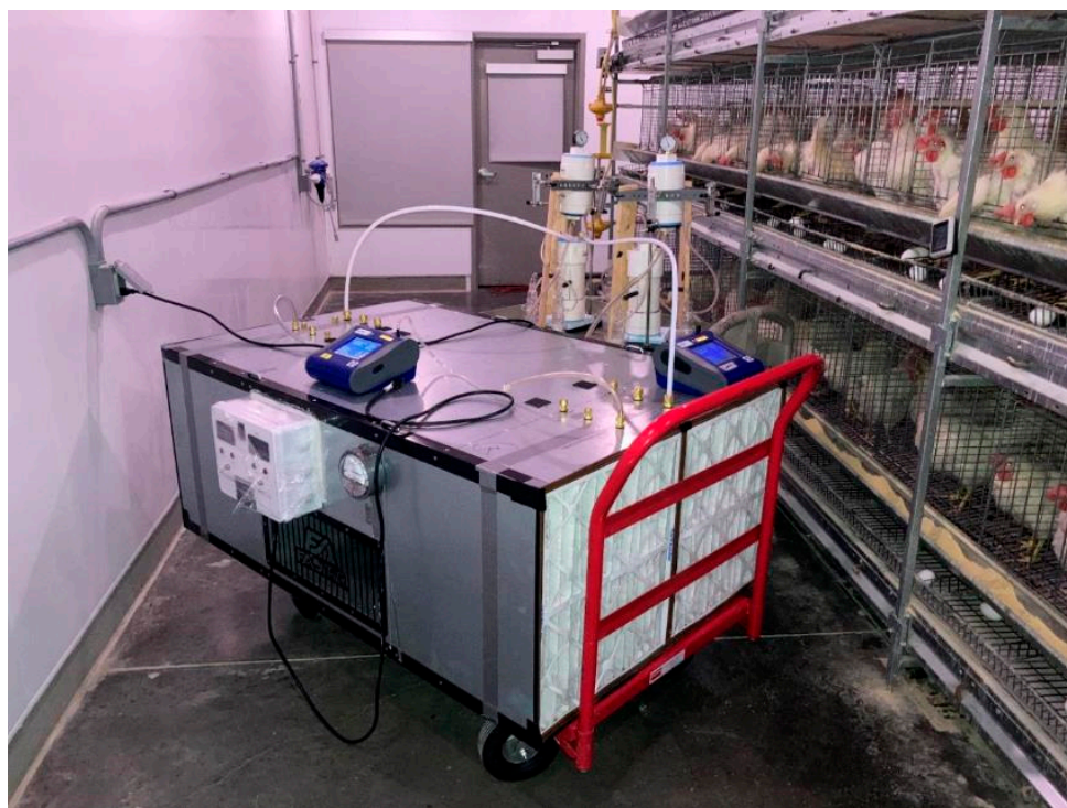
Figure 6. The experimental setup for collecting viable airborne bacteria and PM at a teaching room that housed ~150 laying hens at ISU Poultry Teaching and Research Facility. The red cart was used to deploy the FastAir prototype into the testing room. The brown cart (behind) held all sampling equipment (vacuum pumps, manifolds, and BioSamplers®).
