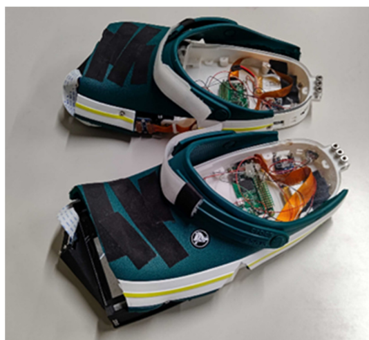
Figure 1. Sensor-integrated clogs for measuring FA and MTC.
