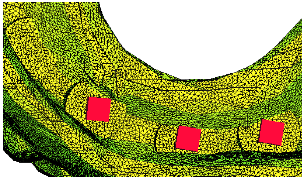
Figure 3. Locking on the surface of three out of four implants.
