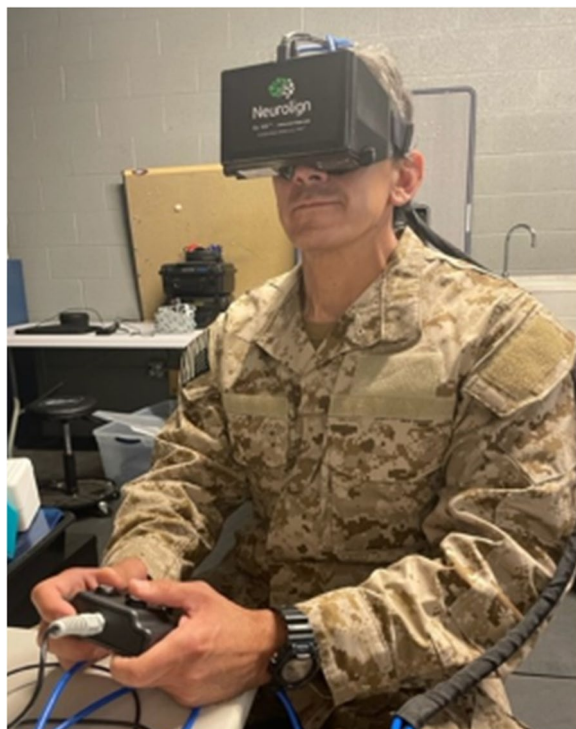
Fig. 2 Eye Tracking Assessment. Legend: A portable head-mounted 3D display system with integrated eye tracking technology measures oculomotor and vestibular function, reaction time and cognitive performance
