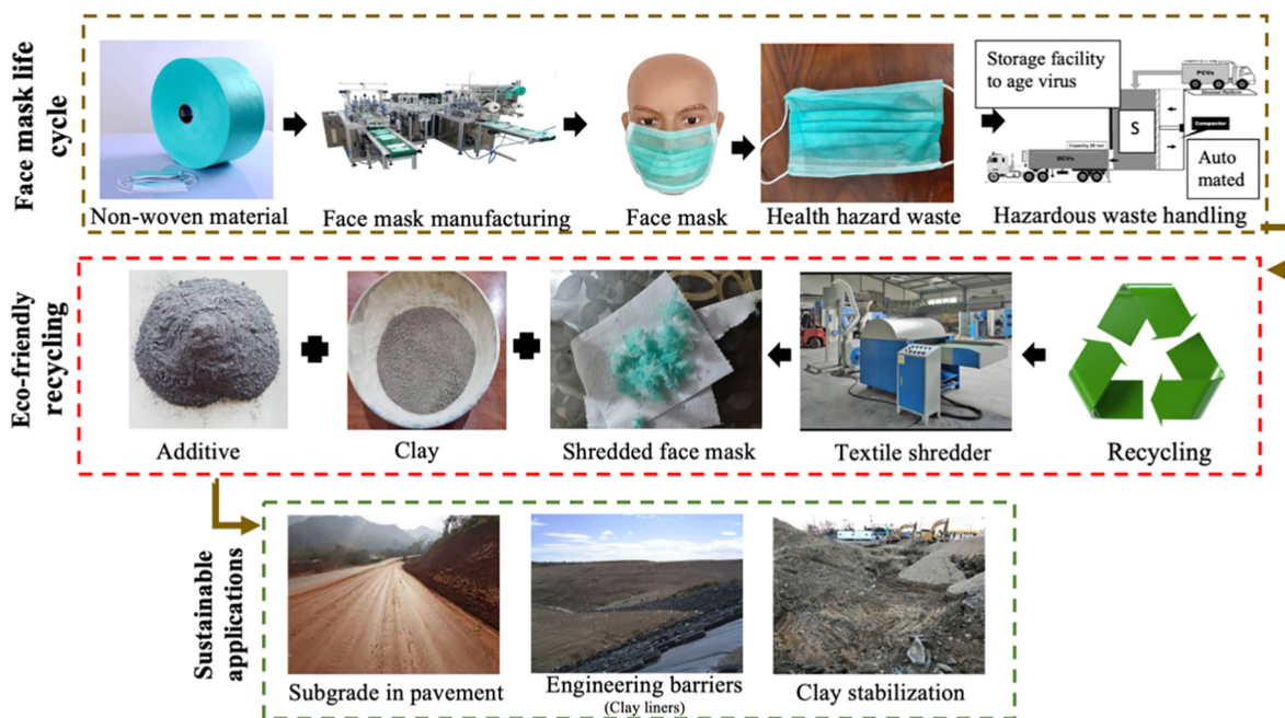
Fig. 5. The recycling flow chart of FM for eco-friendly utilization in Civil engineering projects.
