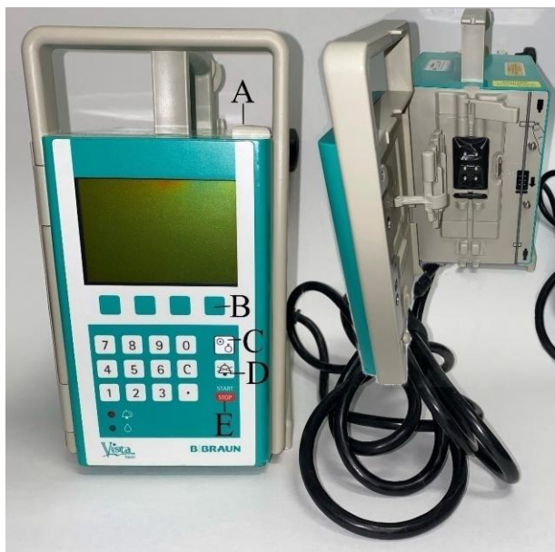
Figure 11. Stationary pump: VISTA basic pump. A , Open door button. B , Function keys. C , On/Off button. D , Silence alarm button. E , Start/Stop button.
