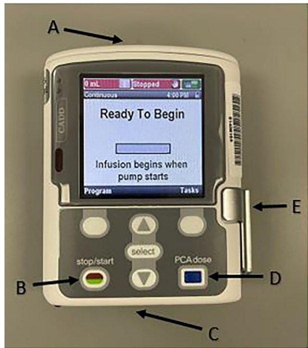
Figure 6. Ambulatory pump (CADD-Solis). A, Battery placement (4 AA batteries). B, Start/Stop function. C, Area of attachment between cassette and pump. D, Bolus dose button used specifically for patient-controlled analgesia. E, Latch for pump connect and disconnect.
