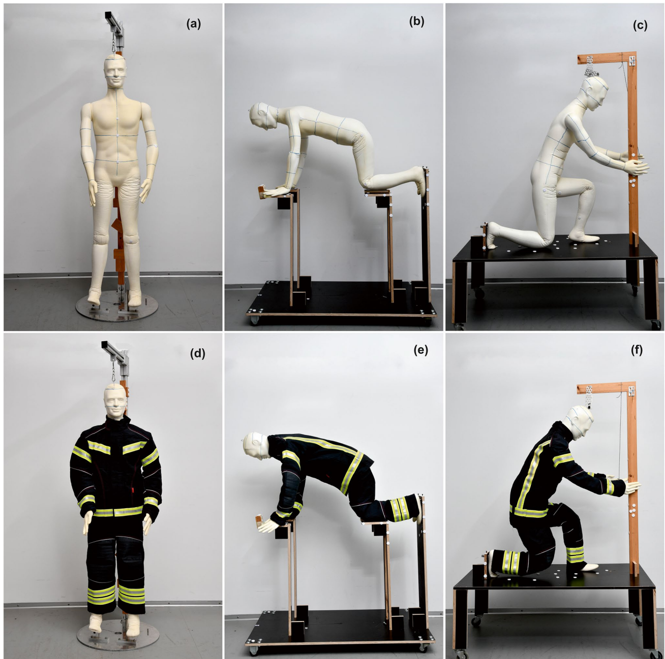
Fig. 1 Body postures analysed in this study including standing upright (a, d), crawling (b, e), and hose-holding (c, f) demonstrated on the nude and dressed agile mannequin fixed to dedicated stands
