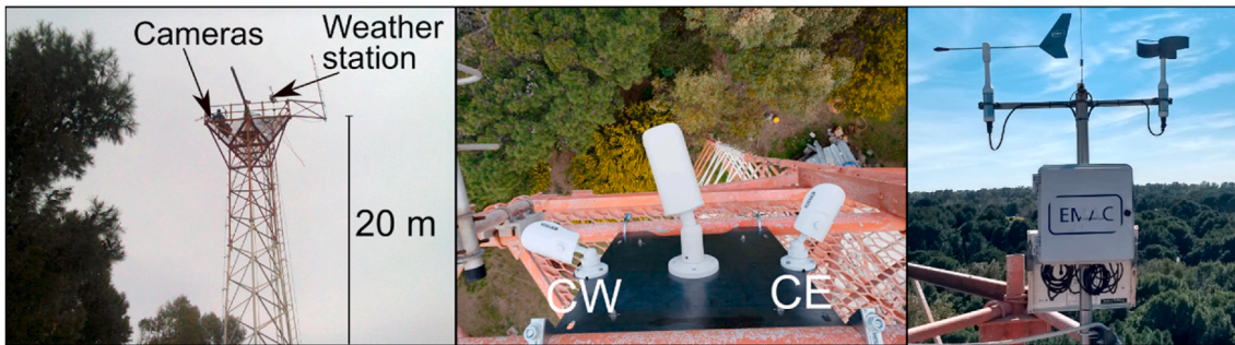
Fig. 2. Coastal Environmental Monitoring Station - EMAC (for its acronym in Spanish). Image A shows the tower in which the EMAC is located; Image B shows the permanent monitoring cameras to the E (CE) and W (CW). Image C is the meteorological station.
