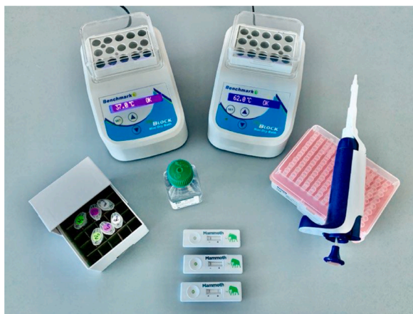
Fig. 3. Minimum equipment required to run the protocol. With appropriate biosafety level 2 requirements, the minimum equipment required to run the protocol following RNA extraction includes Eppendorf tubes with reagents, heat blocks or water bath (37 °C and 62 °C), nuclease-free water, pipettes and tips, and lateral flow strips. Reprinted with permission from Ref. [83]. Copyright 2020 Nature Publishing Group.
