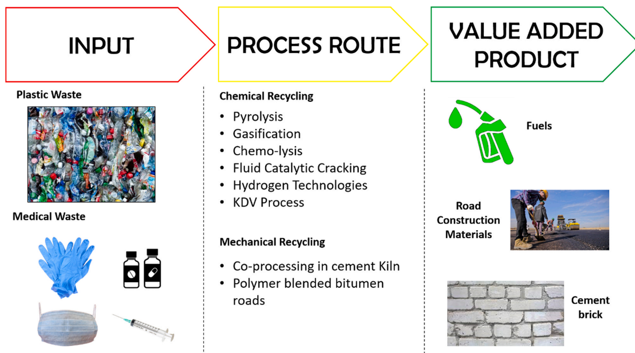
Fig. 4. Comprehensive evaluation of the various process route in converting plastic waste to value-added products.
