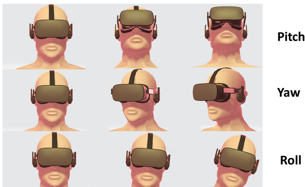
Fig. 1 An HMD user making head movements in pitch (top row), yaw (middle row) and roll (bottom row)
